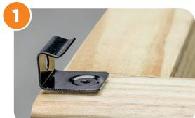
Place a clip on the joist, centered with the cross joist, and fasten with an included screw.
