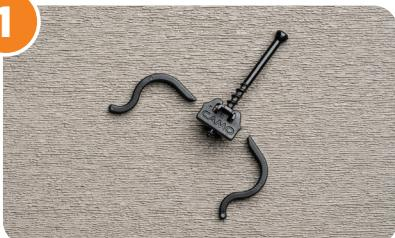
You will need 4 clips for each butt joint. Remove the legs of the EDGE Clips so that they can sit side-by-side on the double joists.
