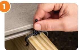
Place an EDGE Clip on the joist with the gusset in the groove. Clips stay in place until you're ready to fasten.
