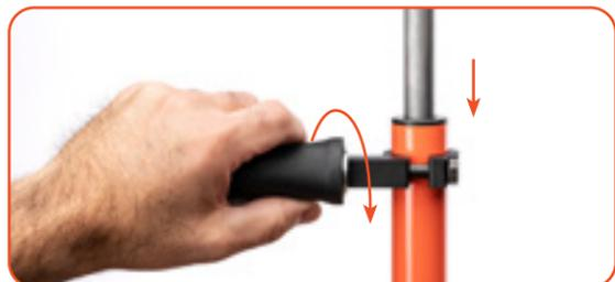
Loosen the handle by turning it counter-clockwise and slide the clamp onto the tool.
