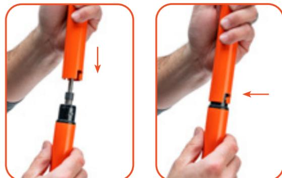
Align the notches in the upper tool body with the locking pins and push down while turning to lock into place.
