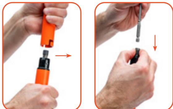
Separate the tool by turning the upper tool body counter-clockwise and sliding the locking pins out of the notches.
